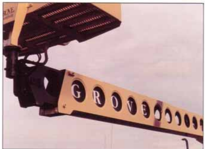
Grove's exclusive trapezoidal boom design provides outstanding rigidity. Side panels feature weight-reducing cutouts with Vierendeel embossing to retain maximum strength.
