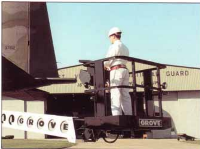
Optional bottom-mount platform with hydraulic rotator provides an additional 3 ft. 7 in. (1.09m) of horizontal reach with no need for extra counterweight.
